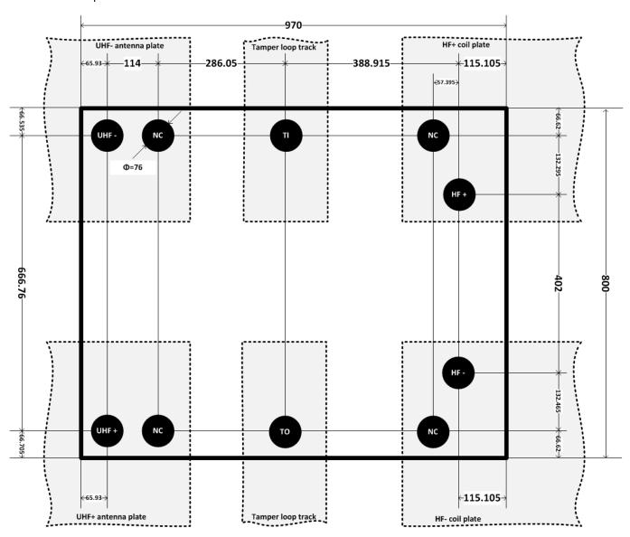
The chip size is calculated including the scribe line. UHF antenna plates and HF coil plates are added here only to illustrate inlay assembly option.
