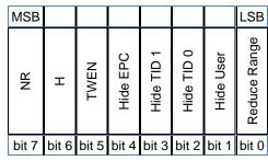
TWEN - used to enable writing of the Tamper Alarm in NVM
